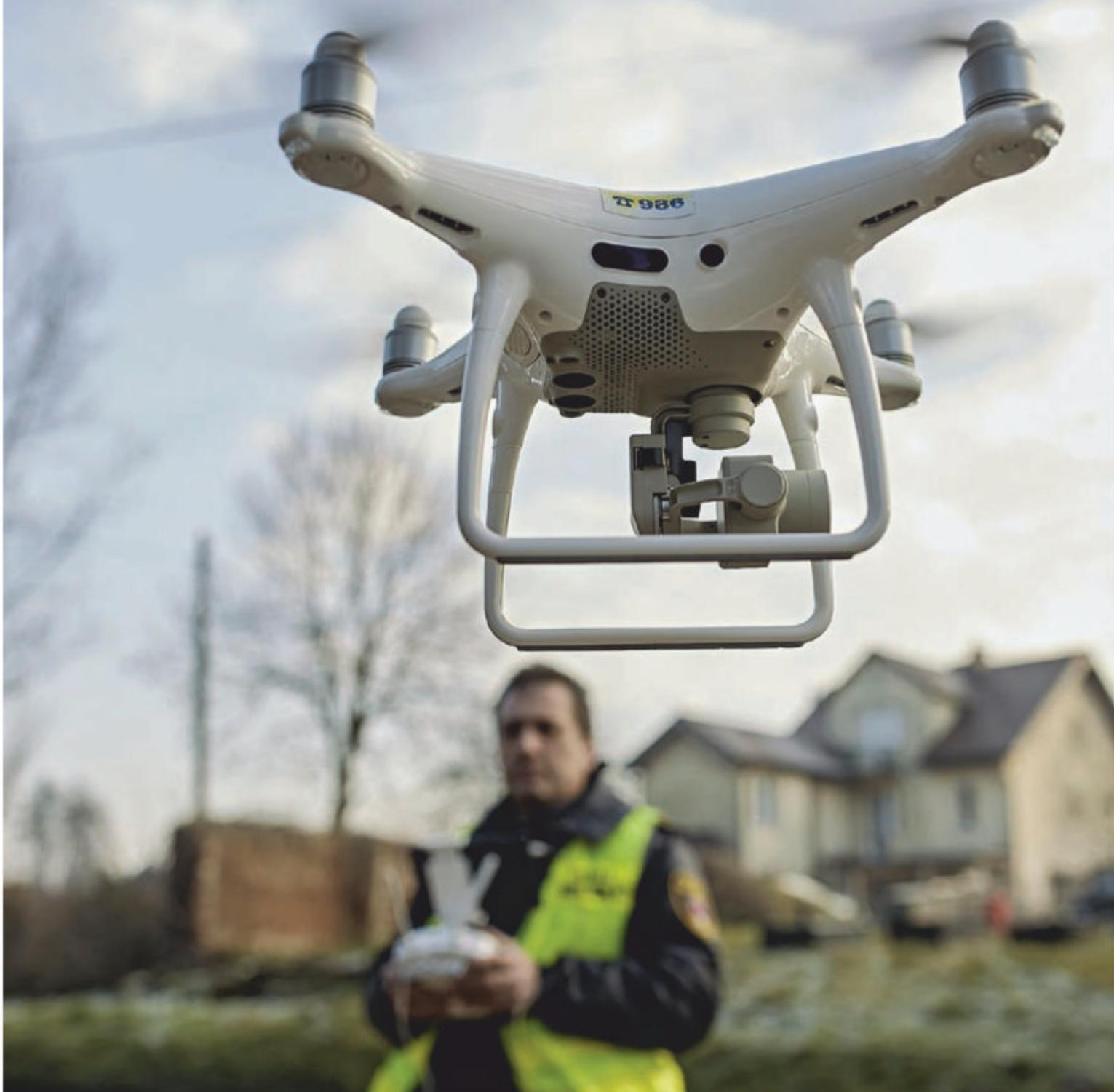
◀ Witkowski's drone checks chimneys for signs that furnaces are illegally burning coal or trash
